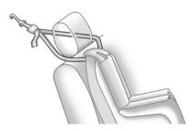
If the position you are using has a fixed headrest or head restraint and you are using a dual tether, route the tether around the headrest or head restraint.
